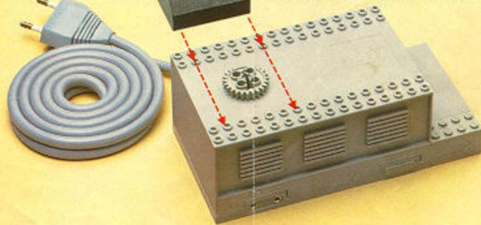
The LEGO® transformer can also be used instead of batteries for LEGO 4.5 volt motors. The control knob **must** be inverted to limit the output to 4.5 volts or you will damage the motor.
