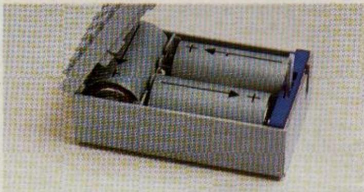
The battery box is opened by loosening the screw in the bottom. When the lid is removed the arrows in the bottom of the battery box show how the batteries are to be placed.
